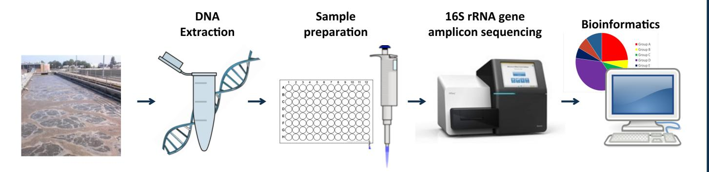
MiDAS<sup>1</sup> provides protocols for DNA extraction, 16S rRNA gene amplicon library preparation<sup>2</sup> and bioinformatic analysis – all optimised for application to wastewater treatment system samples. anaerobic digester organisms have no cultured representatives and are not annotated in popular public databases applied for taxonomic assignment. i.e. the uncultured fermentative bulking filament "*Ca.* Promineofilum" (0092 morphotype).
