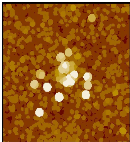
FIG. 13. (Color online) (a): Profile of the silica surface after a simulated impact of a 60 keV \text{Ar}_{12} cluster. Both the initial and the final surface levels are shown. (b): The top view of the same surface. The high areas are shown with lighter shade than the low areas. The surface profile shown in the upper frame represents the area between the horizontal lines. (c): The top view of the surface when analyzed with an “AFM tip” having a 2 nm radius of curvature. Due to the AFM tip convolution effect, the surface profile shown in the upper frame cannot be directly compared with this view.
