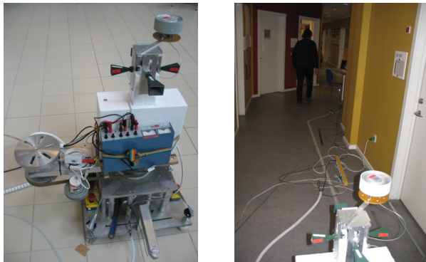
Fig. 1. Left: The pedestal with four horn antennas (three visible) and one omni-directional antenna mounted. Right: The corridor environment.
