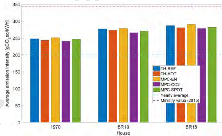
Figure 14: Average carbon intensity for different control strategies for the 3 houses (constant factors from TSO and Energy Agency [55] are provided for comparison).
