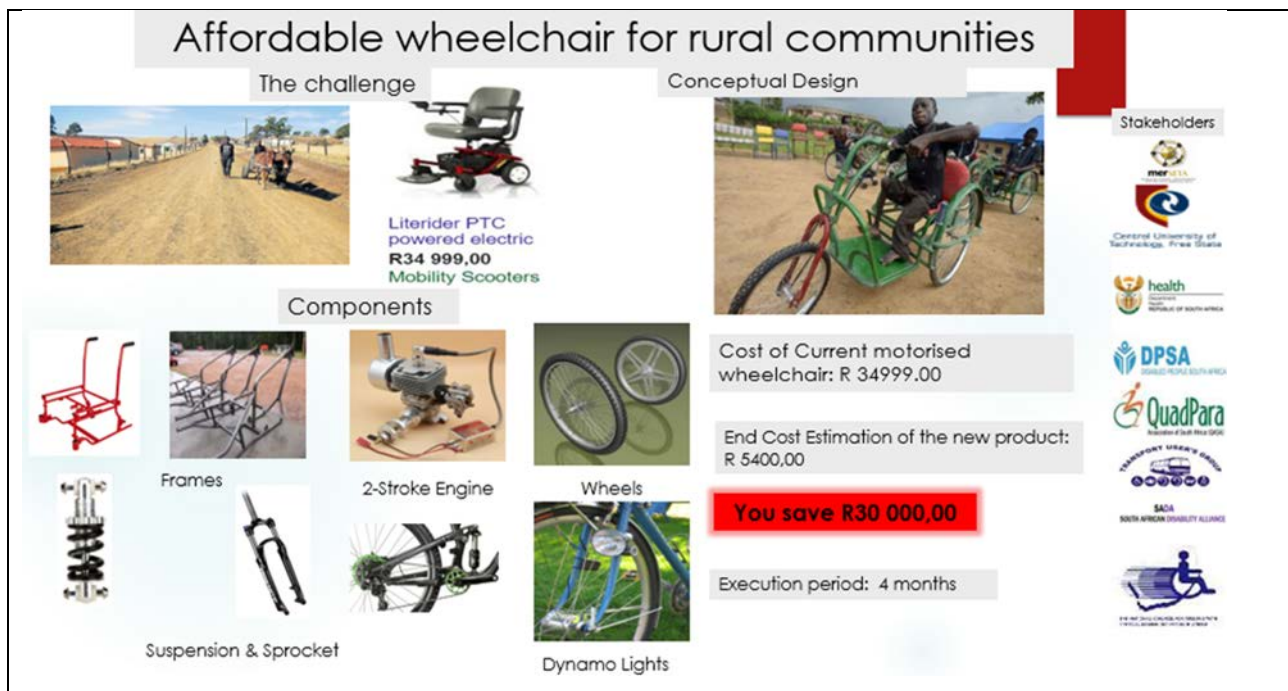
Figure 1: Conceptual design of the affordable wheel chair.
