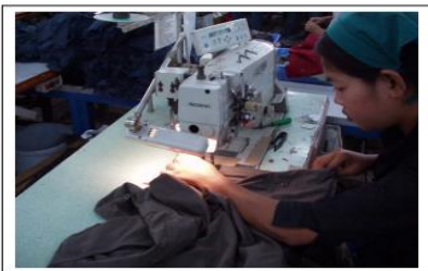
Figure: For close-up work, it is essential to have local lighting where the light shines directly on the task and not into the workers' eyes.
