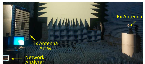
Figure 3. A photo of the measurement setup in the anechoic chamber.
