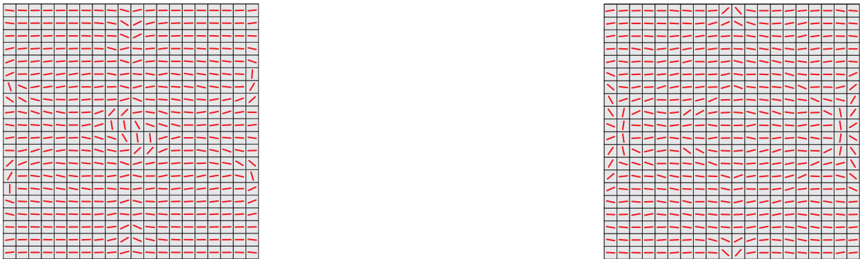
Figure 19: Left: Linear buckling optimized design. Right: General type nonlinear buckling optimized design. The hinged supports are at the left and right edges of the panels.
