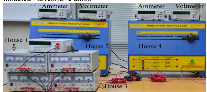
Fig. 11. Hardware Implementation of Scaled down version of DGDSA
