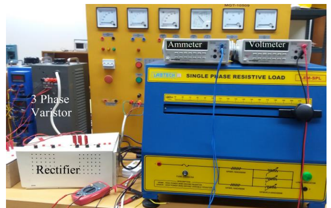
Figure 8. Scaled Down Hardware Implementation for the Calculation of Line Losses and Line Distribution Efficiency
