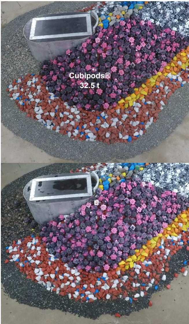
Fig. 8. Front roundhead before testing (left) and after all tests including overload conditions (right).
