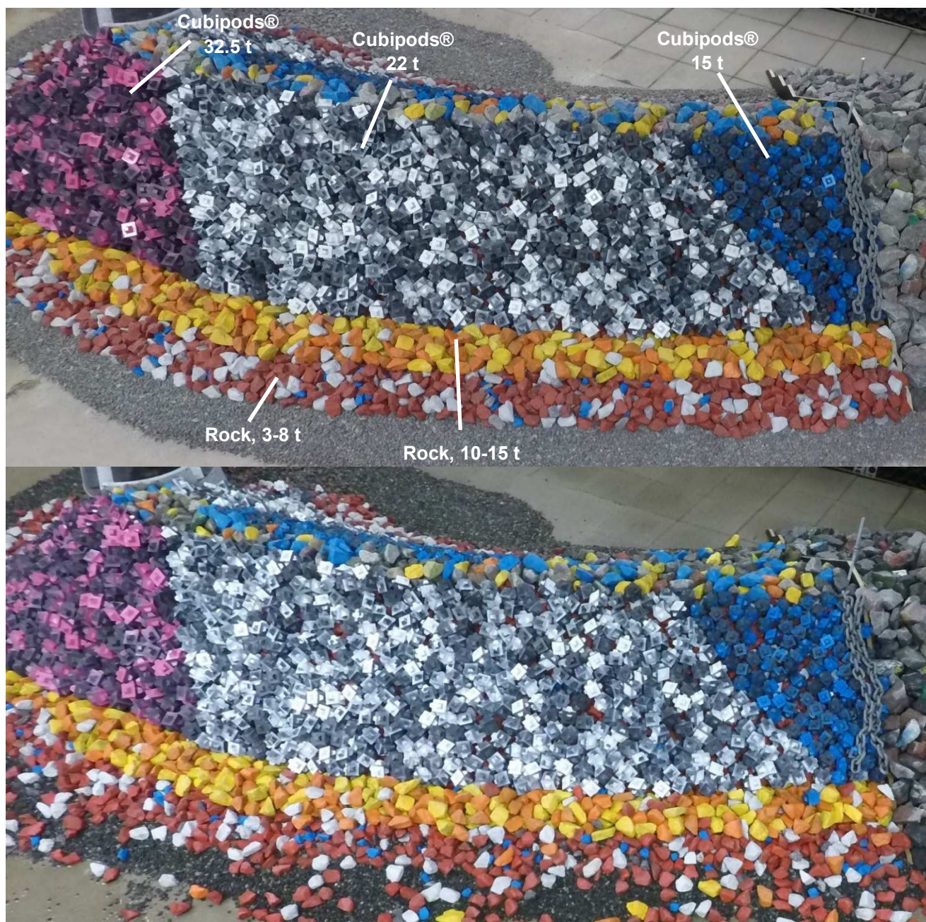
Fig. 6. Trunk section before testing (top) and after overload conditions (bottom).
