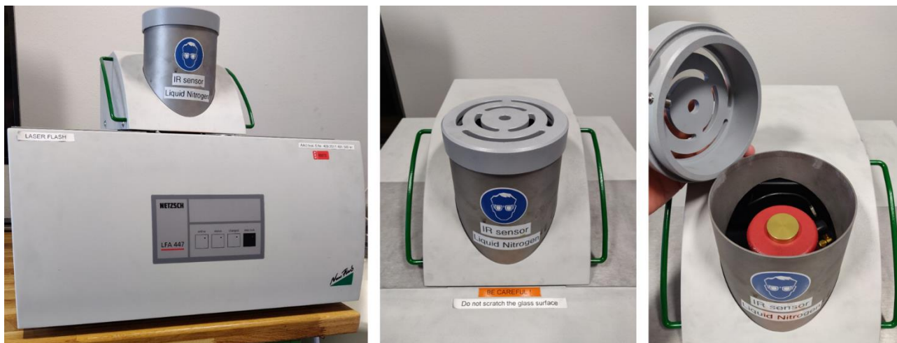
Figure 10: The Laser Flash FLA 447 apparatus (left), the location of the infra-red sensor module on the LFA 447 apparatus (center), removing the top cover (right).
