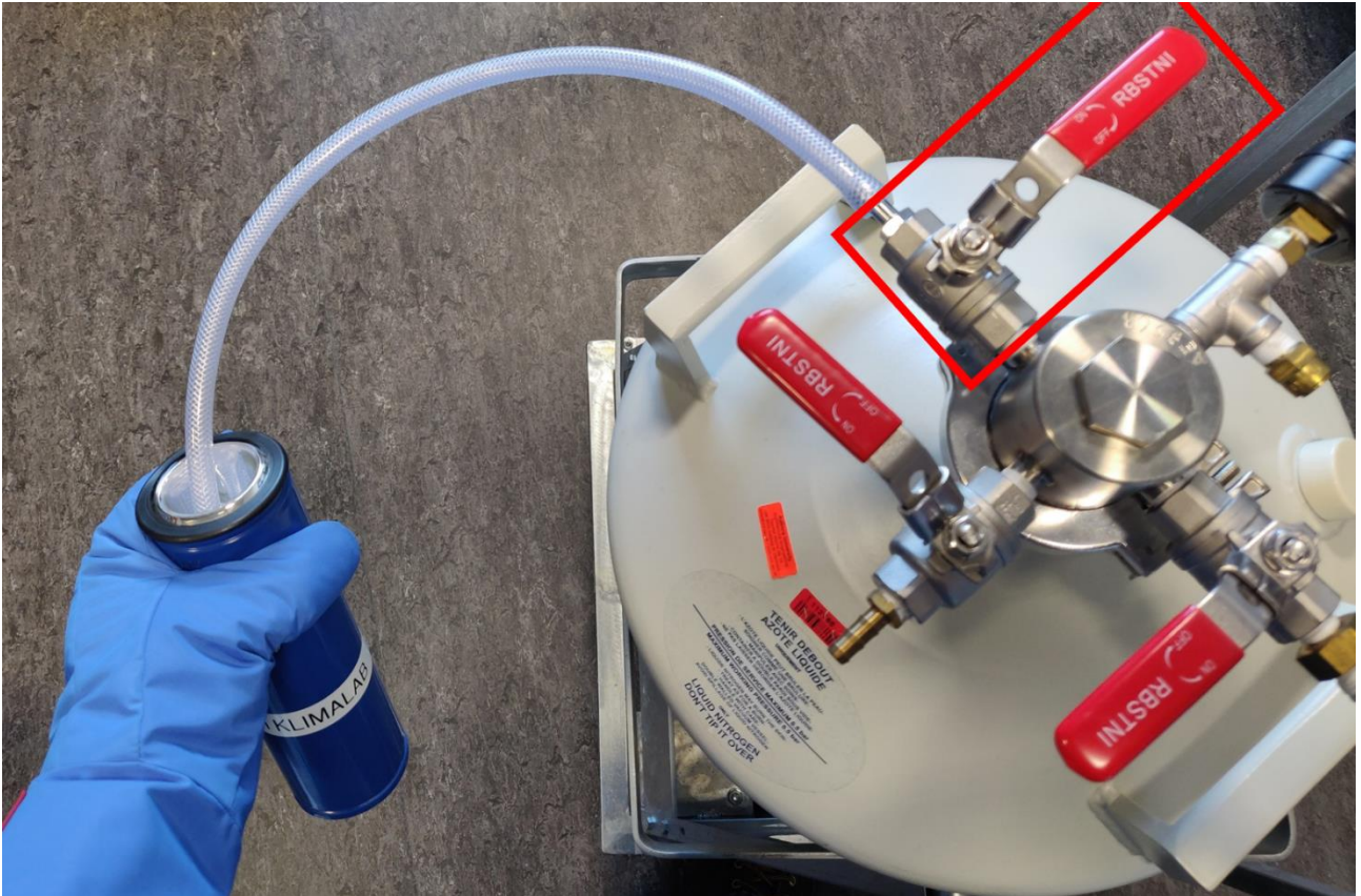
Figure 9: Using the valve connected to the plastic tube to transfer liquid nitrogen into the transfer vessel.
