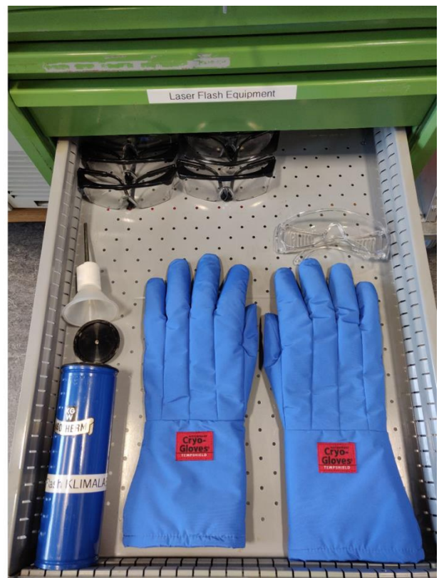
Figure 5: Location of the safety and protection equipment in the dedicated compartment drawer under the Laser Flash apparatus LFA 447.
