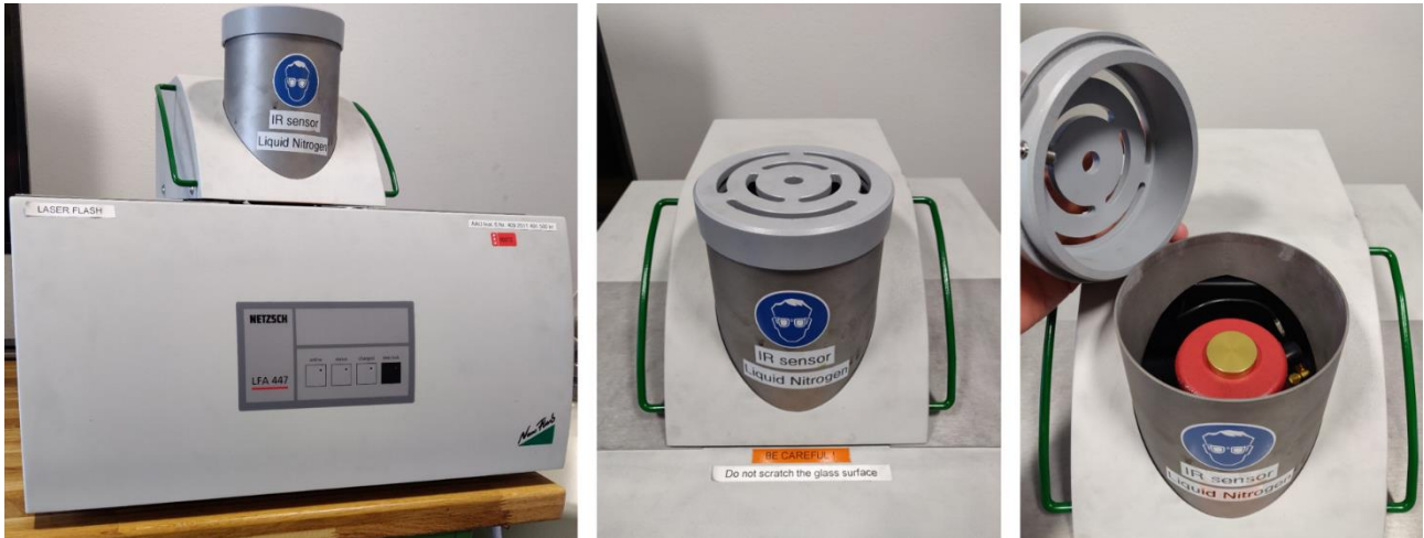
Figure 1: The Laser Flash FLA 447 apparatus (left), the location of the infra-red sensor module on the LFA 447 apparatus (center), removing the top cover (right).
