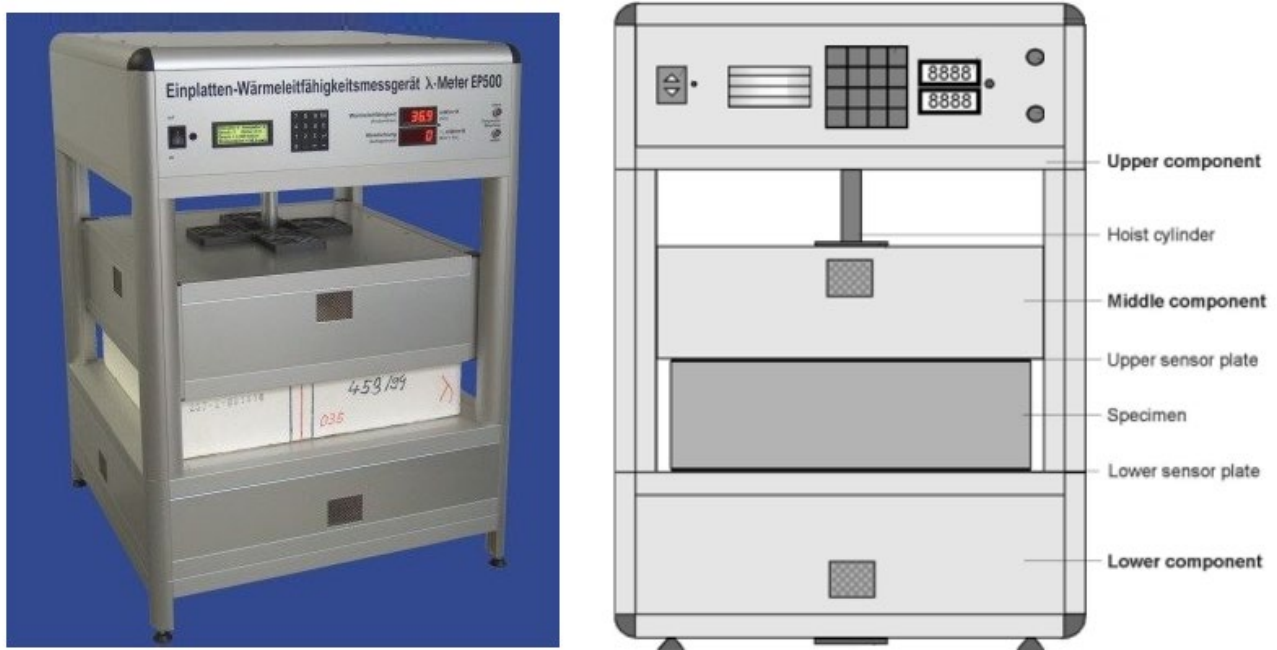
Figure 6: The Guarded Hot Plate apparatus EP500 from Lambda-Messtechnik GmbH Dresden [1].
