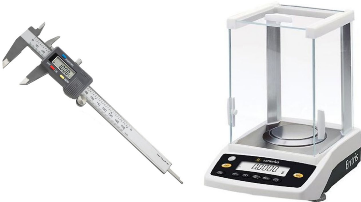
Figure 3: Simple measurement of the material density by measuring the volume (dimensions) and the mass of a sample.
