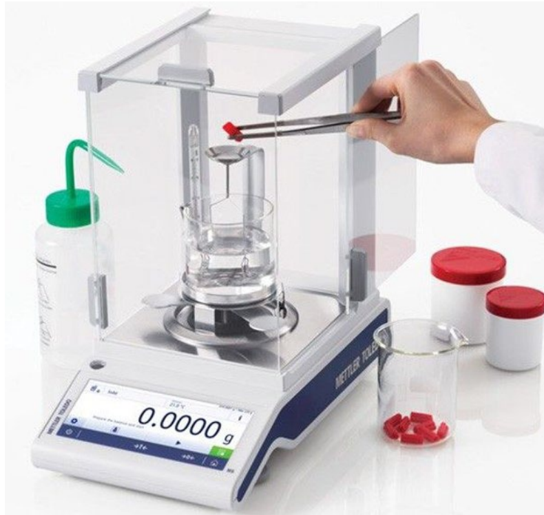
Figure 4: Simple and accurate measurement of the density of a small sample with the Archimedes' principle of buoyancy on a precision scale [2].
