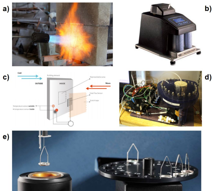
Figure 30: Fire resistance test (a); VSA apparatus for hygrothermal properties measurements (b); In-situ measurement setup (c); ODA 20 for measurement of gas diffusion in porous materials (d); Thermogravimetric Analysis apparatus (e).
