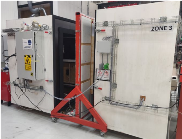
Figure 25: The Guarded Hot Box setup at Aalborg University, Department of Civil Engineering.
