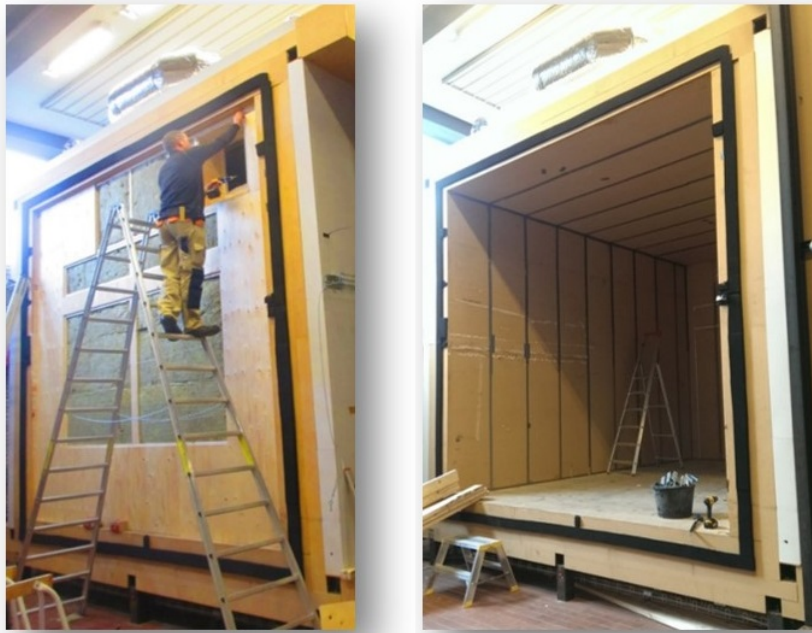
Figure 26: The Big Guarded Hot Box setup at Aalborg University, Department of Civil Engineering.
