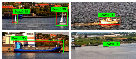
Figure 4: Output of retrained YOLOv3 on optical images
