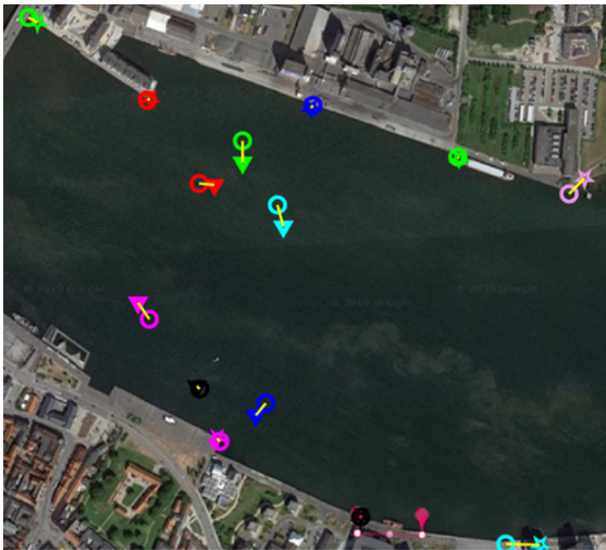
Figure 12: Position estimation test results. Circles represent the true position. Stars and triangles represent the estimated position.
