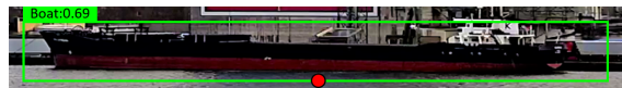
Figure 8: Boat detection indicated by the green bounding box. The red point represents the estimated position of the boat.
