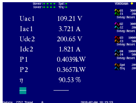
Figure 17. The measured efficiency of the proposed converter when V_g = 110\text{ V} , E = 200\text{ V} , R = 110\ \Omega .
