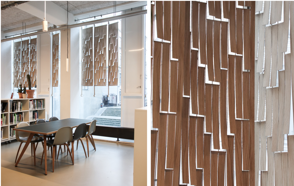
Figure 5 Full scale demonstrator with developed and tested thermal responsive composites in the Copenhagen School of Technology and Design Library. Left image shows the developed composite mounted in operable frames on the glass pane. Right side close-up of the composite bending and creating light permeability through the membrane.
