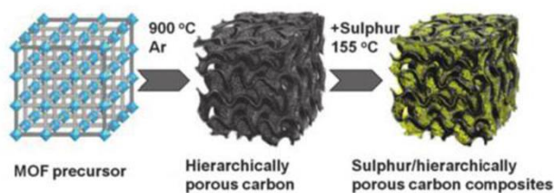
Figure 12. Scheme of sulphur-hierarchical porous carbon composite preparation. [Reproduced from Ref. [129] with permission from The Royal Society of Chemistry.]
