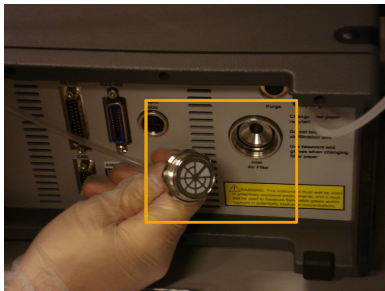
Figure 2. Internal filtration unit.
