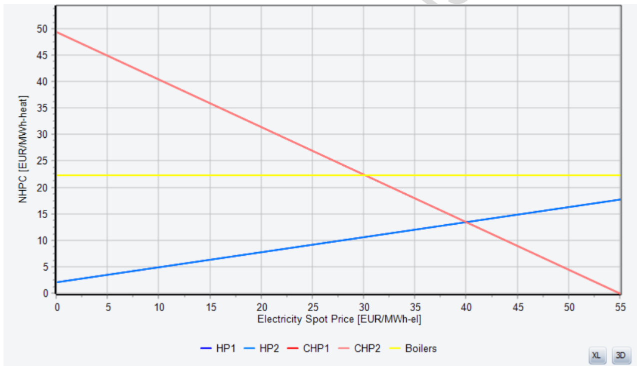
Figure 3: Specific NHPC of the production units as described in section 2, as function of the electricity spot price on the Day-ahead market. Starting costs are not included.
