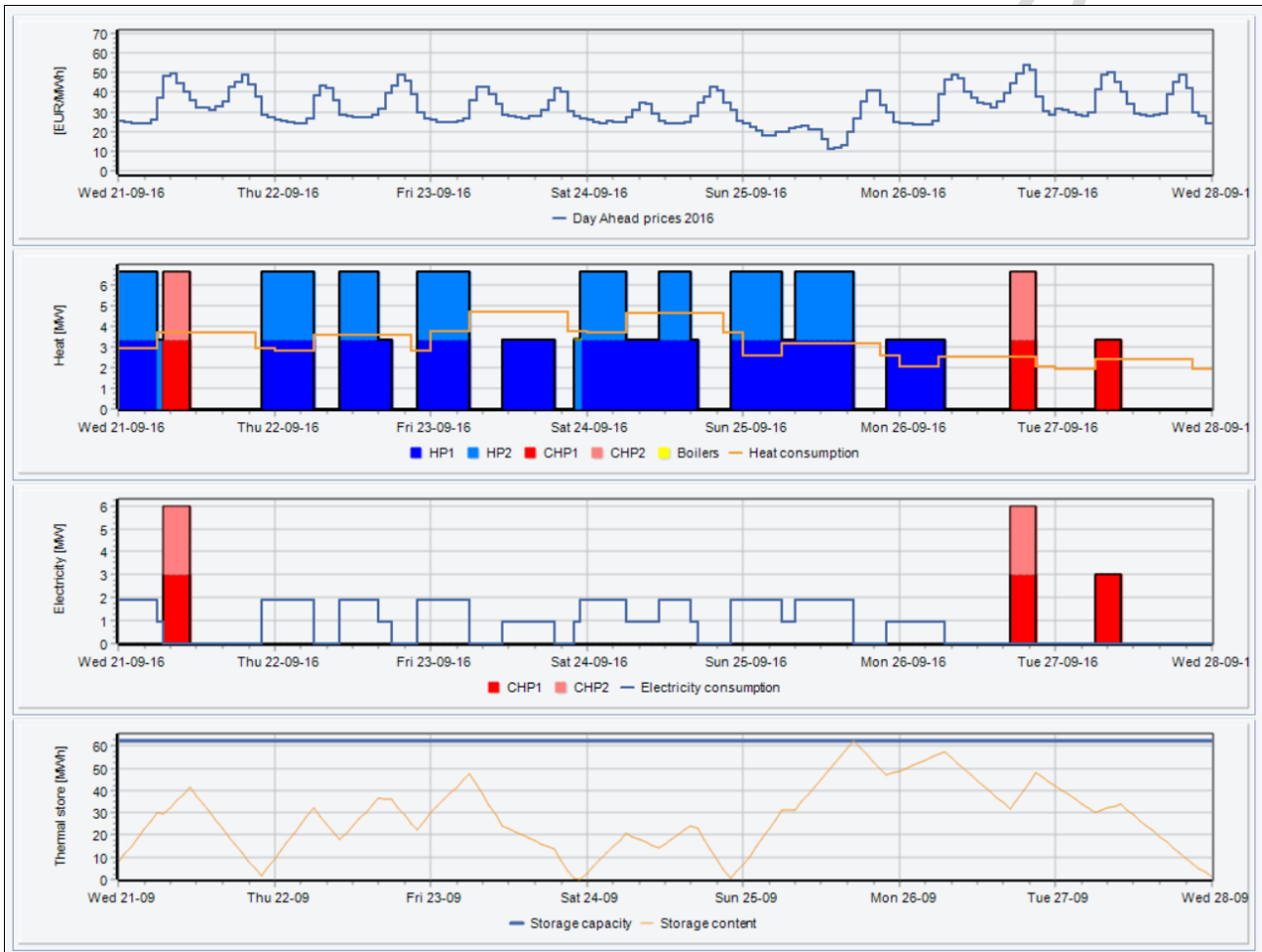
Figure 4: An example of the UC at the DE plant as described in Section 2 during 7 days in September calculated using the advanced analytic UC method.
