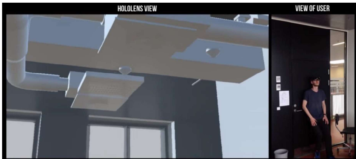
Fig. 1: (Left) AR view of ventilation system in a meeting room. (Right) Viewpoint of the user. This picture is a screen shot from an AR demonstration video from a student project at Aalborg University
