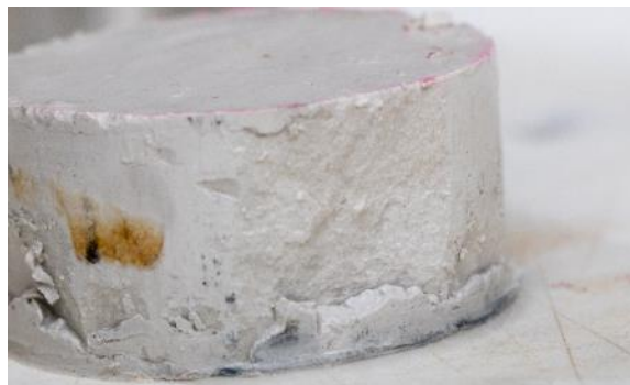
Figure 7 Chalk sample after completed consolidation test. On some parts of the sides, flakes had been broken off during sample preparation.
