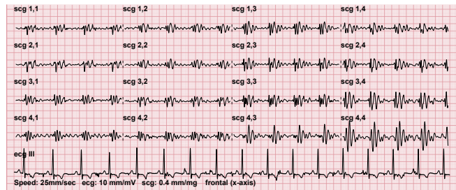
Figure 1 Example of SCG chart for frontal accelerations. Each larger grid square is 5 by 5 mm, which scales to 200 msec and 12.5 mg. Data in figure is from subject 7.
