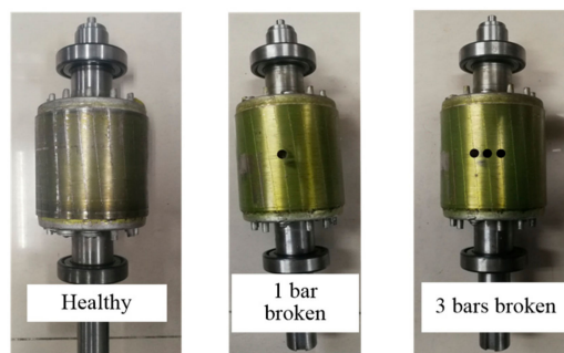
Figure 10. Photos of the Rotors with Holes.
