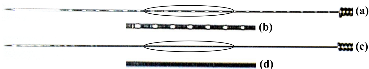
Figure 1. Comparison of acupuncture needles: (a) Nano-SS needle, (b) a higher magnification image taken from the black circle in (a) showing the laser-modified surface feature, (c) U-SS needle, and (d) a higher magnification image taken from the black circle in (c) showing the surface without any modification feature.
