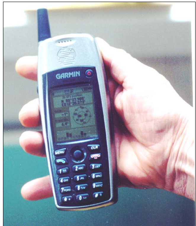
Figure 1: Garmin Navtalk GSM – cell phone, with GPS – was used in the experiments presented in this paper.
