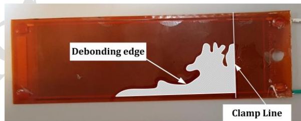
6 7 Figure 10. Debonded area within adhesive and aluminum layer
