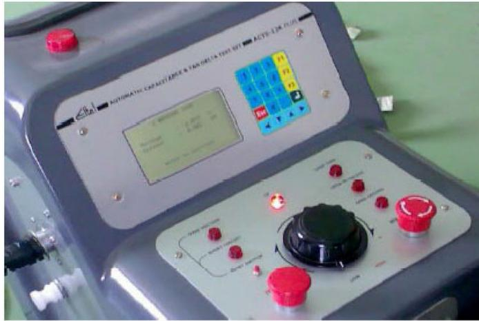
Fig. 1  $Tan\delta$  and capacitance measuring unit
