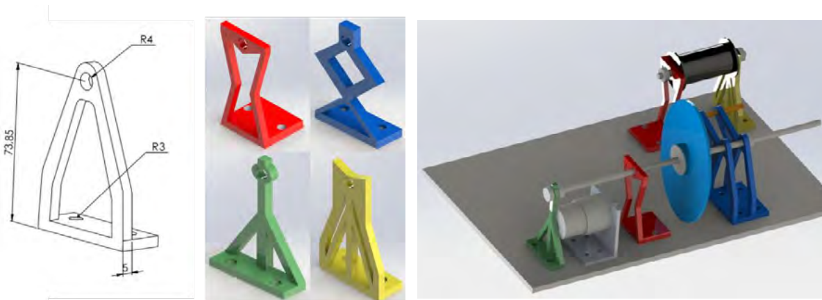
Fig. 3. different CAD models of the slide bearing frames and Solidworks assembly of the winding machine
