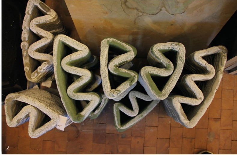
2. Robotically additive-manufactured bricks for the Thermal Tower Project (2018), based on developing thermally-designed concrete composite made through additive manufacturing processes. Photo: MB Jensen (2018).
