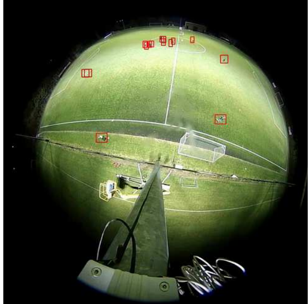
Figure 10: Detections on a test frame. We can note that players are accurately detected, even though there are a few superfluous predicted bounding boxes.
