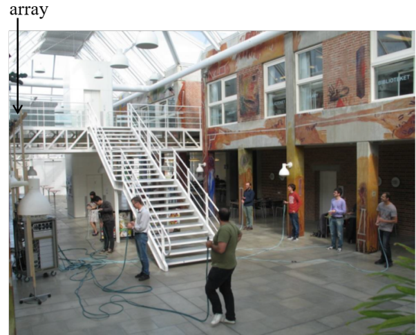
(b) The array is 6 meters long. Eight terminals (y-axis) holding a 2-antenna device are around 2 and 6 meters from the array and move in a square of 1 square meter.
