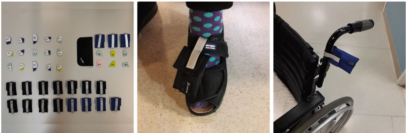
Fig. 5 Left: Overview of bed sensors (top left), resident sensor pouches (bottom), and nurse sensors pouches and RF blocking bag (top right). Middle: Resident wearing sensor on foot. Right: Sensor placement on resident’s wheelchair
