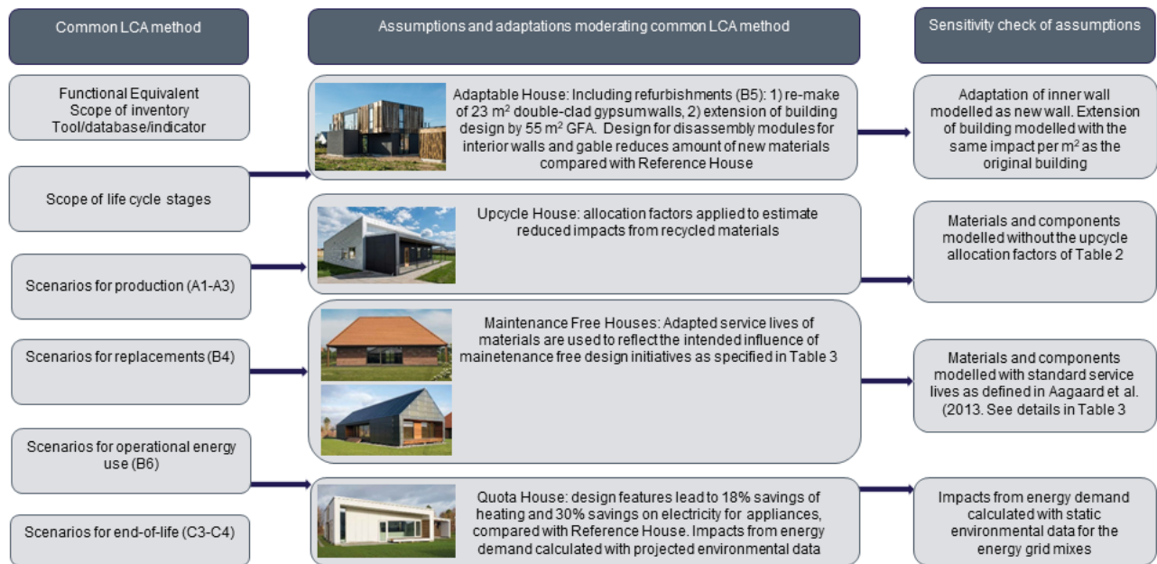
Figure 1. The methodological set-up of current study: The common LCA method, the adaptations/assumptions and the sensitivity check of these assumptions.
