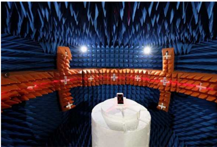
Figure 1.13: MPAC anechoic chamber for FR1 MIMO OTA testing.
