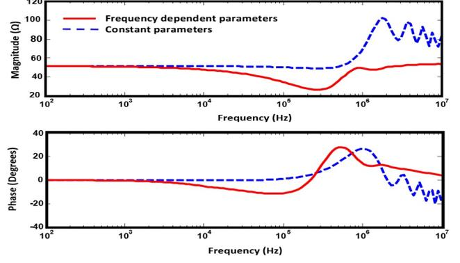
**Figure 6:** Input impedance of the vertical electrode of length  $l = 24$  m. Red solid line: frequency dependent model and blue dashed line: constant parameters model.  $\rho_0 = 1000 \text{ } \Omega \cdot \text{m}$ ,  $\epsilon_r = 10$ .
