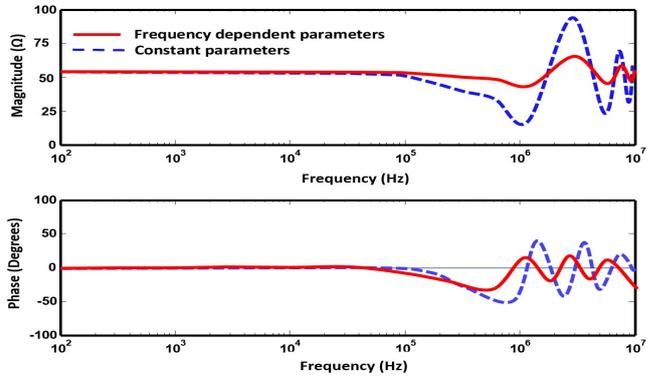
**Figure 10:** Input impedance of the vertical electrode of length  $l = 12\text{m}$  which is buried in two layer soil,  $\rho_{01}=100 \Omega\cdot\text{m}$ ,  $\rho_{02}=1000 \Omega\cdot\text{m}$  and  $\epsilon_r=10$ . Red solid line: frequency dependent model and blue dashed line: constant parameters model.
