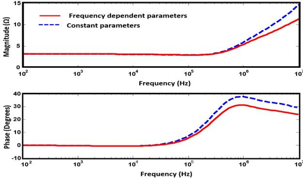
**Figure 4:** Input impedance of the vertical electrode of length  $l = 3$  m. Red solid line: frequency dependent model and blue dashed line: constant parameters model.  $\rho_0 = 10 \text{ } \Omega \cdot \text{m}$ ,  $\epsilon_r = 10$ .
