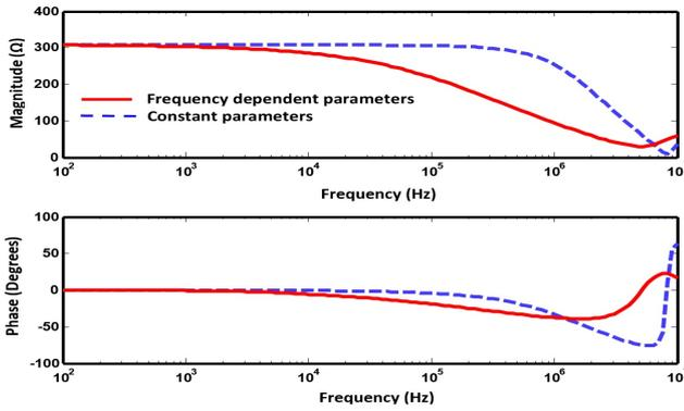
**Figure 5:** Input impedance of the vertical electrode of length  $l = 3$  m. Red solid line: frequency dependent model and blue dashed line: constant parameters model.  $\rho_0 = 1000 \text{ } \Omega \cdot \text{m}$ ,  $\epsilon_r = 10$ .
