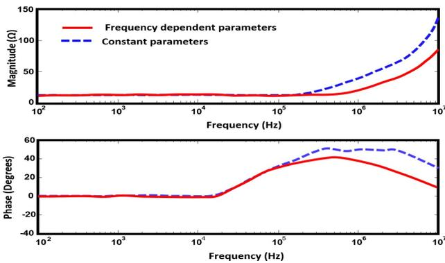
**Figure 8:** Input impedance of the vertical electrode of length  $l = 3\text{m}$  which is buried in two layer soil,  $\rho_{01}=100 \Omega\cdot\text{m}$ ,  $\rho_{02}=1000 \Omega\cdot\text{m}$  and  $\epsilon_r=10$ . Red solid line: frequency dependent model and blue dashed line: constant parameters model.
