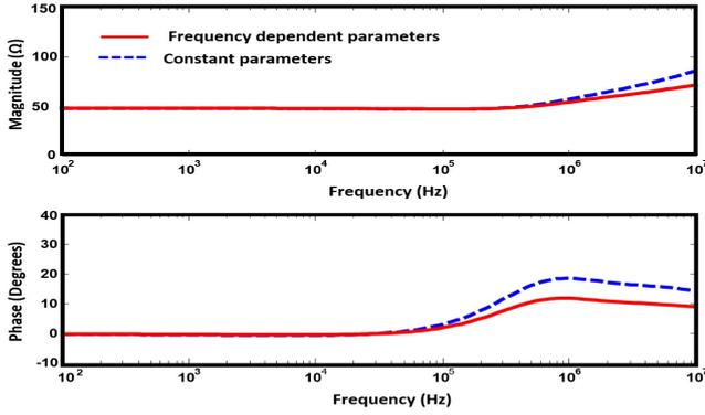
**Figure 7:** Input impedance of the vertical electrode of length  $l = 3\text{m}$  which is buried in two layer soil,  $\rho_{01}=1000 \Omega\cdot\text{m}$ ,  $\rho_{02}=100 \Omega\cdot\text{m}$  and  $\epsilon_r=10$ . Red solid line: frequency dependent model and blue dashed line: constant parameters model.
