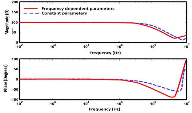
**Figure 9:** Input impedance of the vertical electrode of length  $l = 12\text{m}$  which is buried in two layer soil,  $\rho_{01}=1000 \Omega\cdot\text{m}$ ,  $\rho_{02}=100 \Omega\cdot\text{m}$  and  $\epsilon_r=10$ . Red solid line: frequency dependent model and blue dashed line: constant parameters model.
