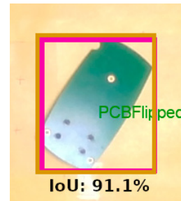
Fig. 7: An example of the IoU score of the PCB in one of the test images. The prediction is illustrated with a purple rectangle while the ground truth with a brown one.
