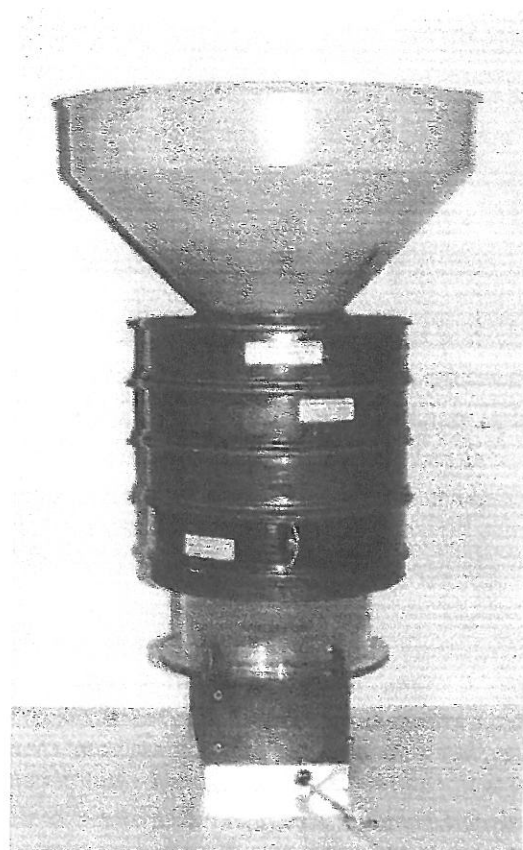
Fig. 9. Funnel placed on top of the sieves. The sand is filled into the funnel after the weight of the sand has been measured. The same amount of sand is used each time. (Photo No 27).
