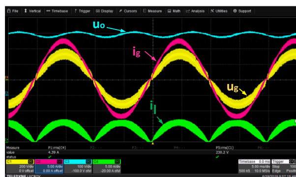
Figure 14. Measured waveforms of two units interleaved using parameters ( f_{sw} = 20 kHz) and a phase shift of 180° given in Table 5.
