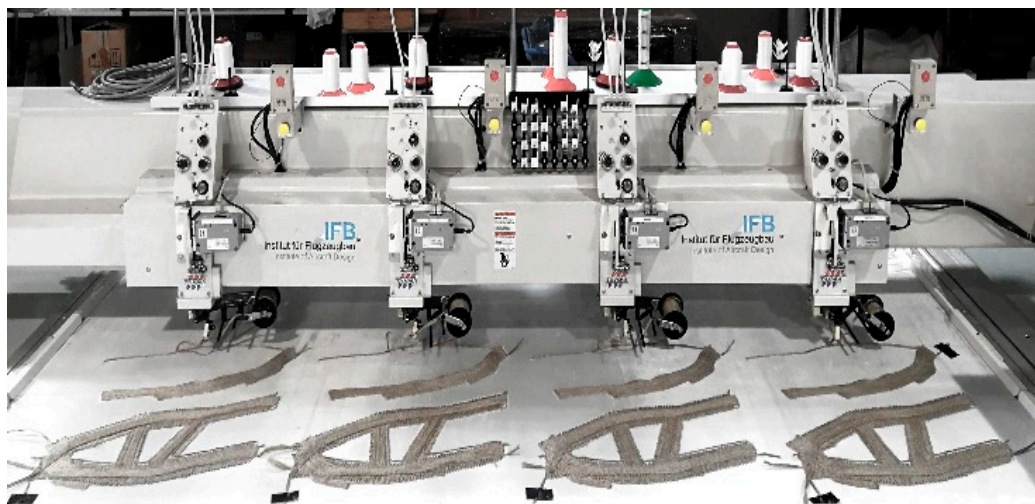
Figure 8. Fabrication with 4-head embroidery Tajima TFP machine, provided by IFB.
