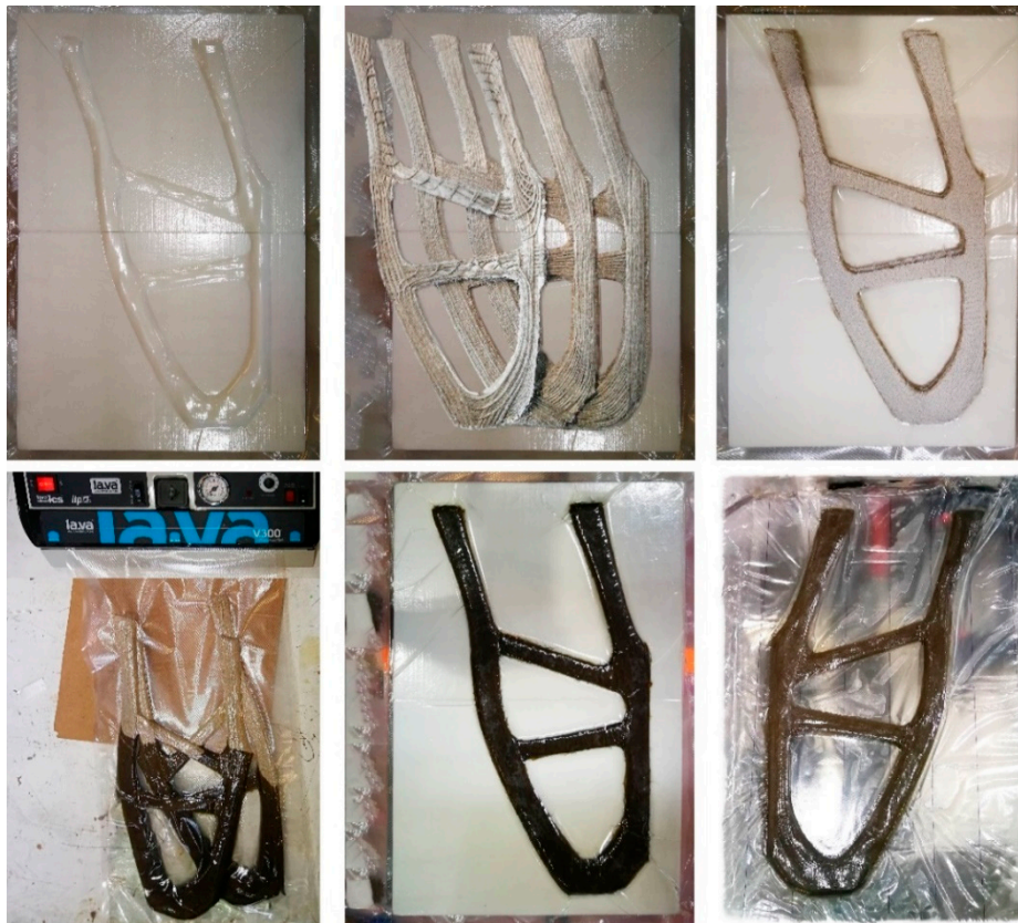
Figure 9. Mold and laminate preparation using airtight sealing bags, resin infusion and vacuuming 292 of stapled laminate layers, demolding at IFB (counterclockwise from top left to bottom right).
