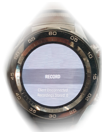
Fig. 3. Main view of QCApp running on a WearOS device. It contains a button for starting and stopping the on-spot quality inspection process: "Record"; information about the connection with the computer: "Client Disconnected"; information about how many audio and acceleration are stored in the memory of the watch: "Recordings stored: 0".
