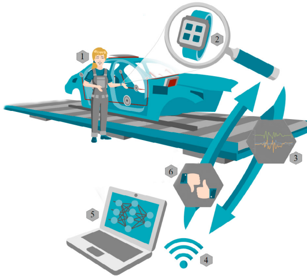
Fig. 1. Framework structure: 1. The worker is performing the assembly action; 2. The smartwatch is gathering data while the action is performed; 3. Data is sent to the computer for processing; 4. The connection between the smartwatch and the computer is made through the local wireless network; 5. The received data is classified using AI on the computer; 6. The classification result is sent to the smartwatch and the feedback for the performed action is given to the worker.
