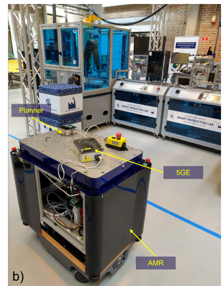
Figure 11. (a) Architecture of the 5G-integrated MEC AMR planner solution including the AMR, WMAGW, 5G network infrastructure, and AMR fleet manager controller and planner deployed in edge-cloud configuration. (b) Picture of the 5G-integrated MEC AMR planner solution deployed for 5G emulation at the lab.
