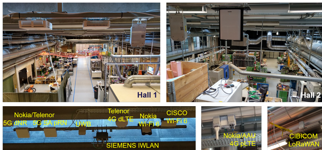
Figure 2. Overview of the Aalborg University 5G Smart Production Lab, including details on the two industrial halls and the different operational wireless network deployments.
