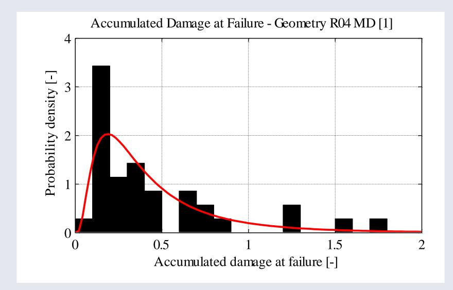
For the reference uncertainties listed above a partial safety factor for the material properties  $\gamma_m$  equal to 1.37 is calibrated using an annual reliability index equal to  $\beta$ =3.09. This corresponds approximately to the total partial safety factor 1.38 used in IEC 61400-1.
