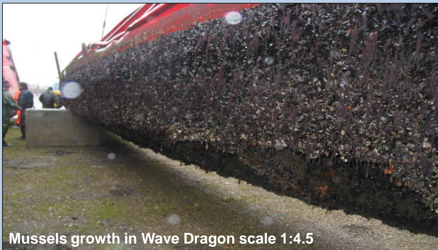
Mussels growth in Wave Dragon scale 1:4.5
