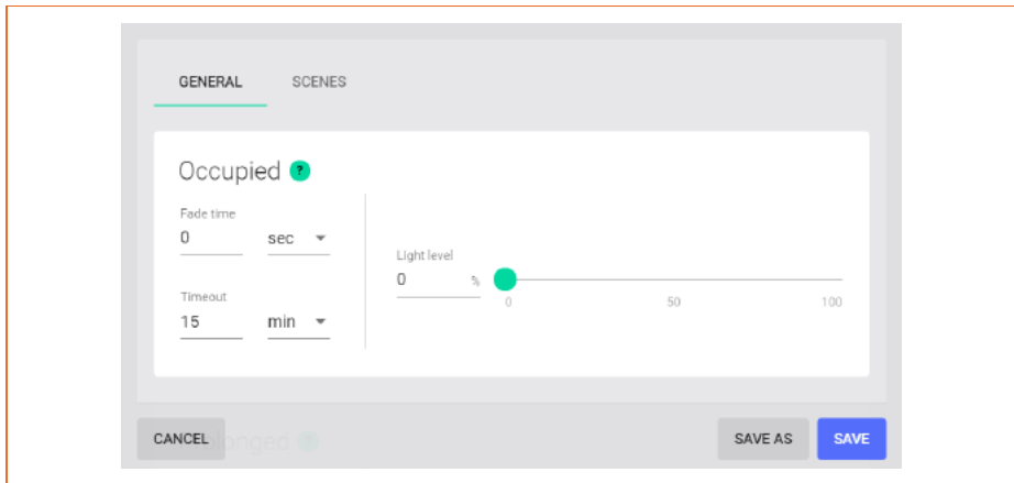
Figure 3: Setup to turn off UV lights when occupancy is detecting via the Silvair Web App
