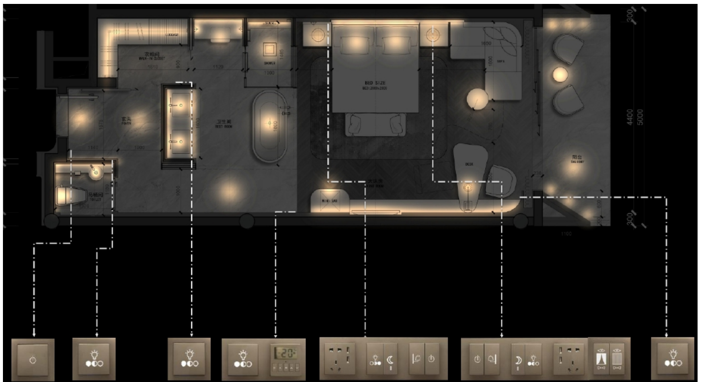
Figure 7: Chinese Five-star hotel's king room lighting layout rendering and lighting control panel
