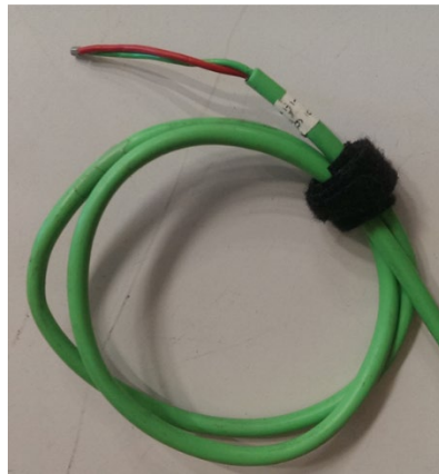
Figure 12: A formed sensing/measurement junction on a type-K thick thermocouple.
