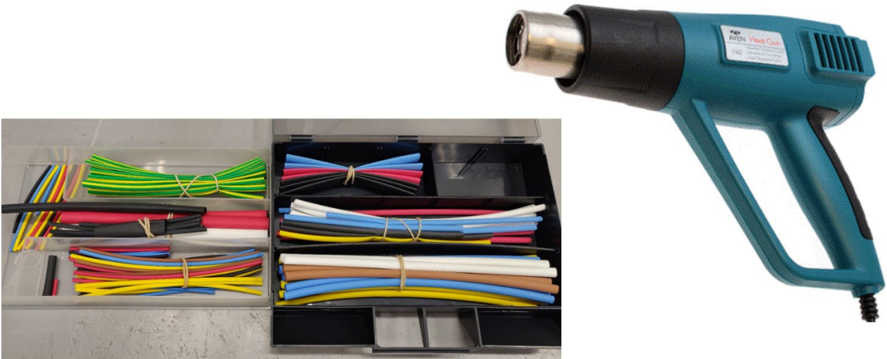
Figure 26: Colored thermo-shrinking ring (left) and heat gun to shrink the rings (right).
