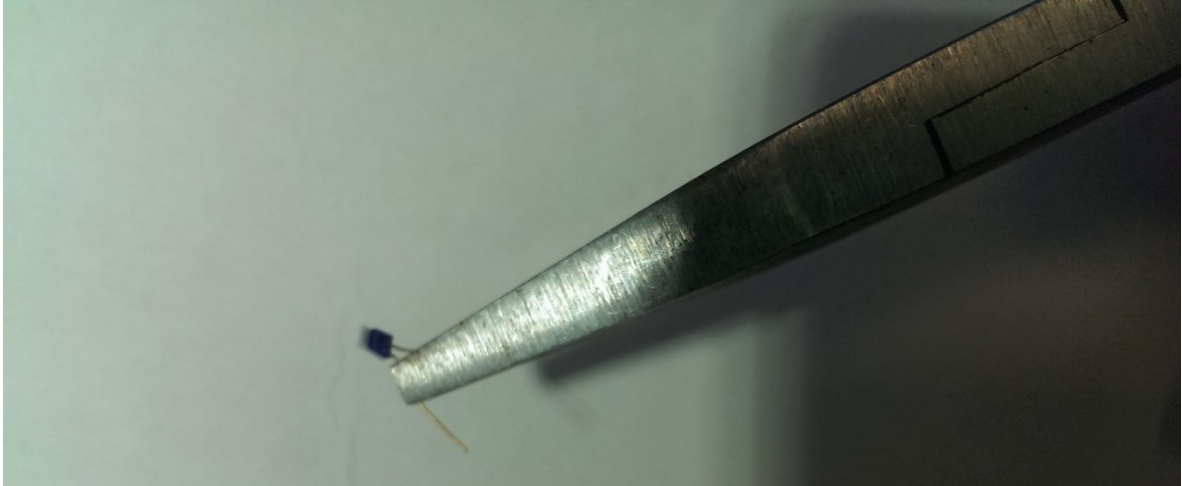
Figure 30: Holding the leg of the Pt 100 that will be connected to the long side wire. The leg that is inserted (in contact with molten tin) is the one held by the plier and not the other one.
