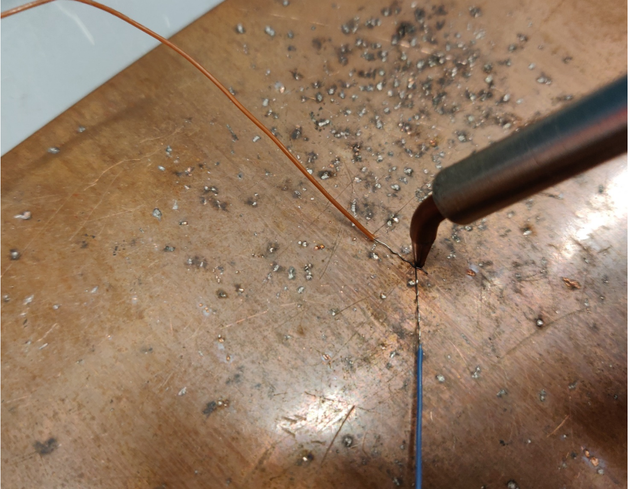
Figure 6: Welding a thermocouple as a single-point-of-contact junction with an electrical welding tool.
