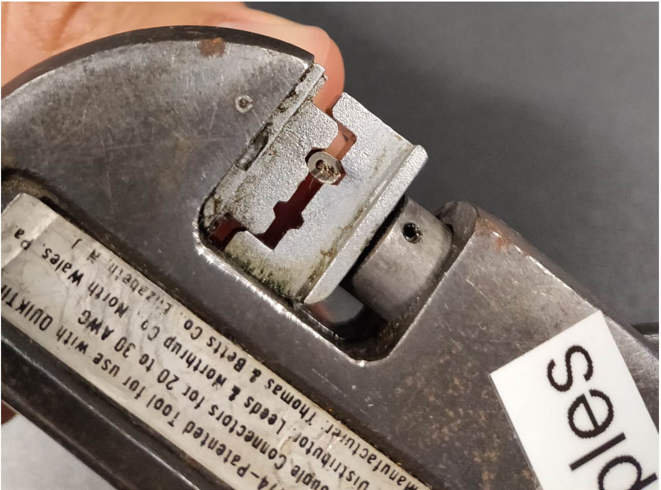
Figure 10: Pressing the pressure connector on the type-K thermocouple to form the sensing/measurement junction.
