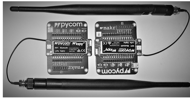
Figure 6. Pycom/LoPy4 micropython enabled microcontroller and 868 MHz antenna, used to create LoRa nodes.
