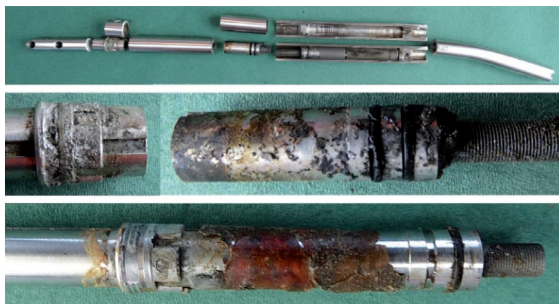
Figure 8. Examples of a sectioned STRYDE (top panel), corroded bushing (middle panel), and presence of biological material on internal components. Biological origin was verified with EDS analysis showing a high oxygen content (bottom panel).
