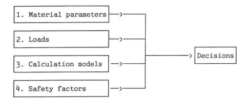
The four components are of equal importance and have to be introduced in a code. Safety factors are often embedded in calculation models. Safety margins are the gap between the ultimate limit state and the serviceability limit state.
