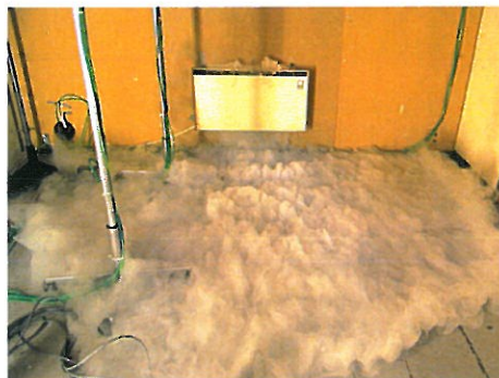
Figure 2. Development of stratified semi-radial jet from the ULV device.
